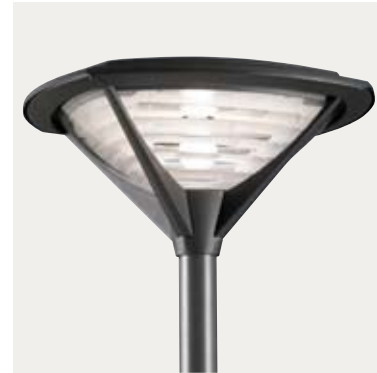
Logo (FSM/SE/ST/MT) Rotation symmetrical optics with UV-resistant plastic design louvres. A metal anti-glare shield is positioned around the lamp burner.
