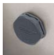
Gore™ filter Provides the balance of the internal/external pressure and eases the expulsion of humidity condensation.
