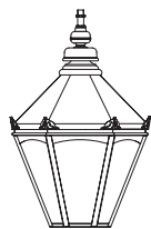
Suspended mounting Threaded spigot type, 1 inch Gas (Ø 34 pdg)
